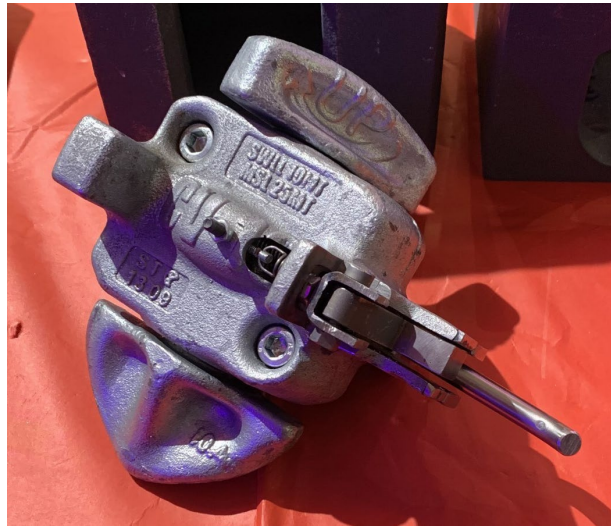
Figure 4. Assembled lock without lock shaft in unlocked position.
