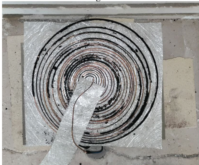
Figure 1. The single-wire copper coil positioned on a steel sheet with glass fiber in-between for insulation.
