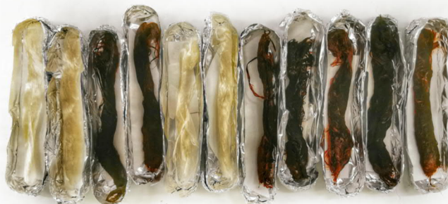
Figure 2 Ioncell® fibers are made of cellulose and cellulose-lignin blends. At a glance, fibers dyed with a darker color contain lignin in different amounts. In this illustration, each Ioncell product is laid in an aluminum tray.
