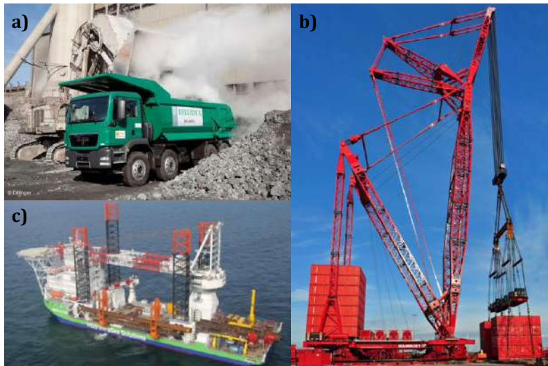
Figure 2.2. Examples of applications of High Strength Q/Q&T steels (a) Wear resistance steel plates used in dumpers (b) Heavy weigh cranes and (c) Offshore rig-legs.
