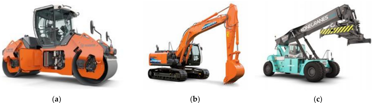
Figure 15. Off-highway vehicles with energy recovery systems. (a) Wirtgen-Group tandem roller. (b) Hitachi excavator. (c) Konecranes reach stacker. [116,124,125].
