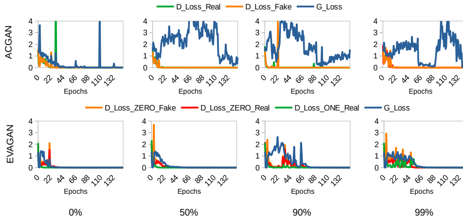
Figure 7. CV GANs losses: The training losses on train set for ACGAN and EVAGN for MNIST dataset in different undersampling scenarios. The upper limit to the loss has been fixed to 4 for the sake of consistency to highlight the difference.
