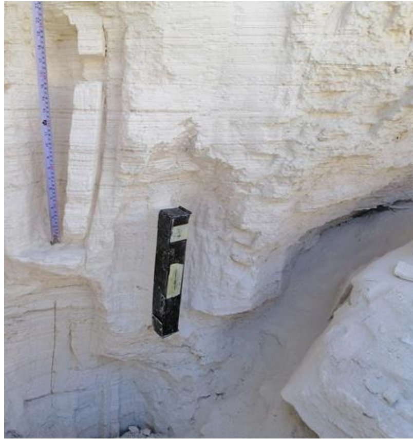
Figure 3.4 DS1 section laminated sediments sampling. Shown is the lower part of the section and the custom made sampling box (5 x 5 x 35 cm) used for the sampling procedure.
