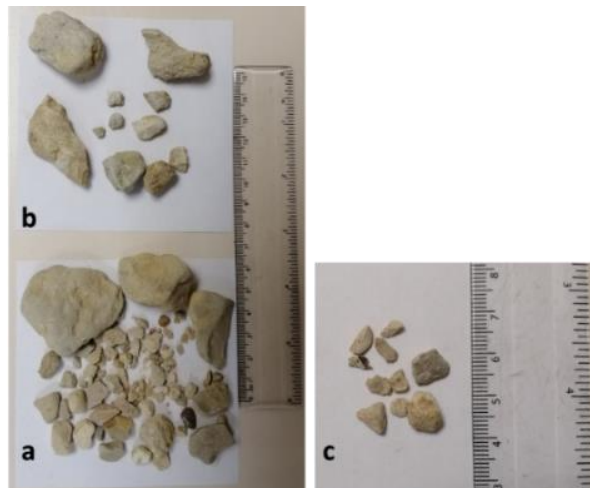
Figure 5.6 Loose sediments of the gravel fraction in the Gh lithofacies beds of the GH1 section. a) Base bed, b) Bed at 0.44 m from base, c) Upper bed at 3 m above base.
