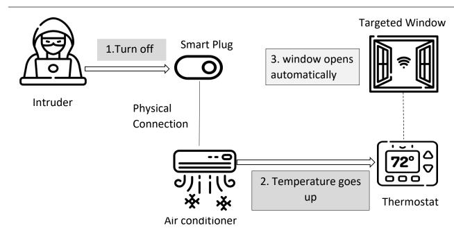
Figure 1. Intrusion due to device interdependence.
