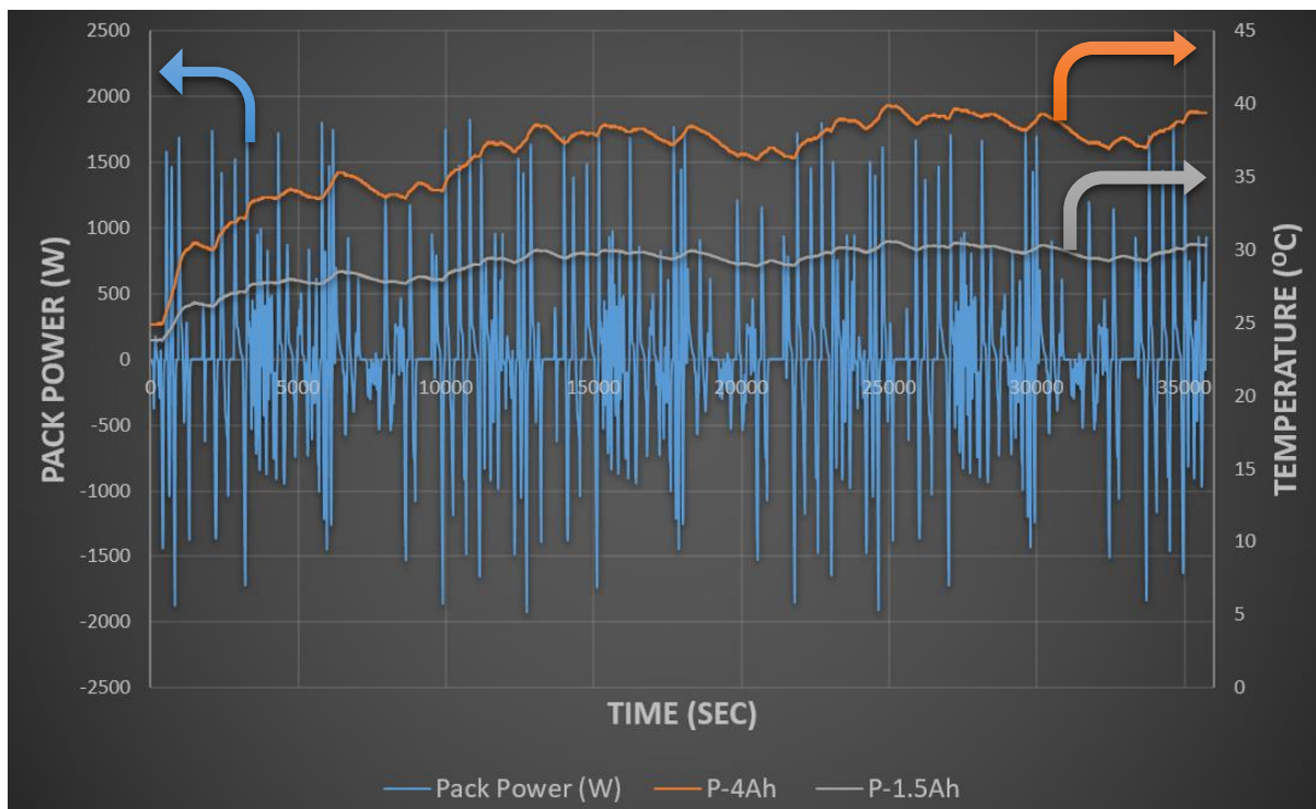
Figure 20. Real world drive cycle result showing temperature profiles (in °C) of P-4Ah and P-1.5Ah corresponding to Pack Power profile (in W) as a function of time (in sec).
