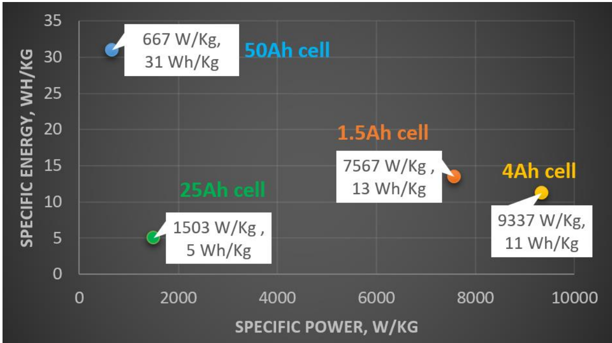
Fig. 10. Specific energy vs specific power for 50Ah, 25H, 1.5Ah and 4Ah at MaxC only during discharge phase.
