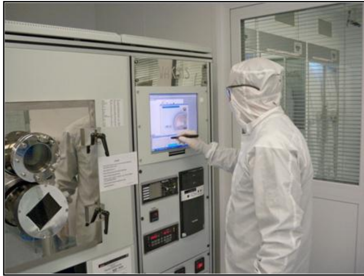
Figure 4.2 Thermal Evaporator, Vaksis PVD Vapor – 3S. Picture taken from [40].
