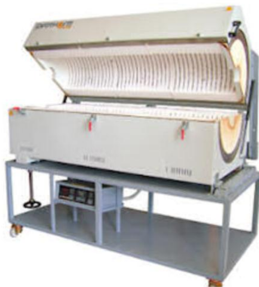
Figure 4.6 Quartz tube furnace used for post-deposition annealing. Image taken from [44].
