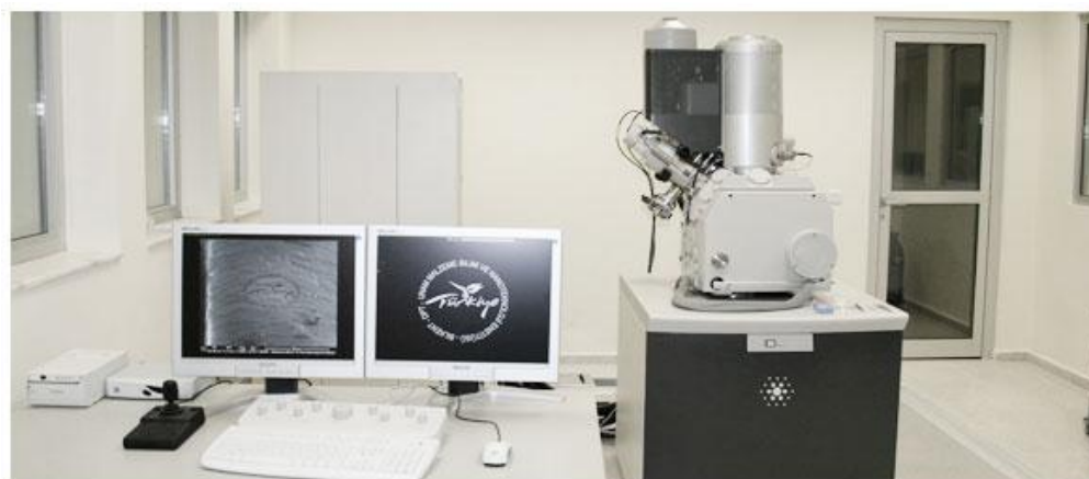
Figure 4.10 The FIB instrument used for the experiments presented in this thesis (FEI Nova 600i Nanolab). Picture taken from [47].
