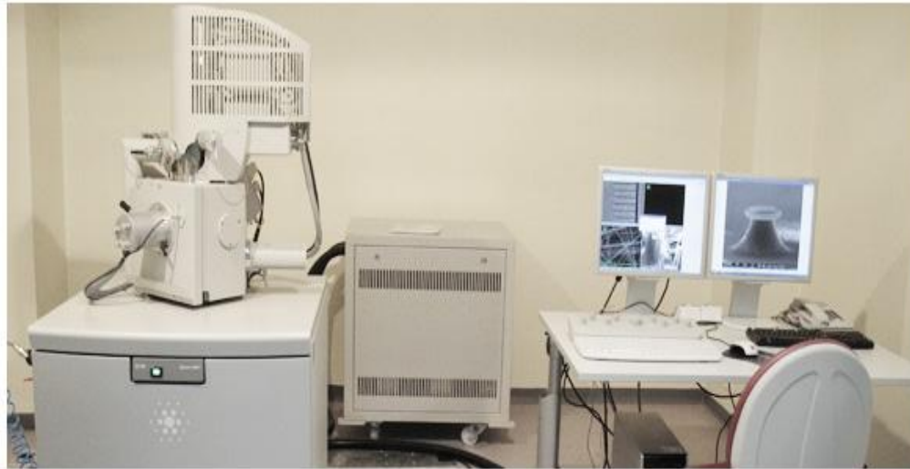
Figure 4.3 The SEM instrument used for the experiments presented in this thesis (FEI Quanta 200 FEG). Picture taken from [42].
