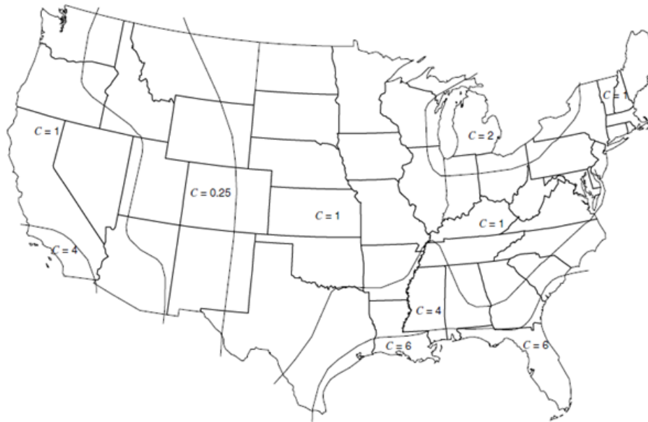
Figure 2.1: Barnett-Vigants atmospheric propagation conditions map for the United States.
