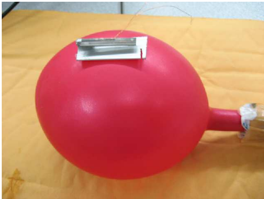
Figure 5.17: Heart Phantom with z-shaped bimorph attached
