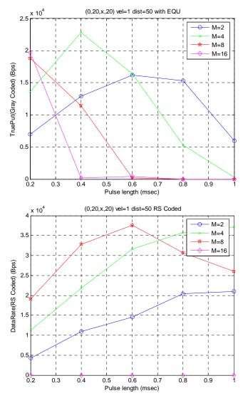
Figure 5.35: Trueput and RS coded data rate performance of the diver scenario#2 and boundary state scenario#1 with Doppler shift (v=1 m/sec) with respect to OFDM pulse length
