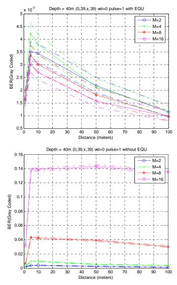
Figure 5.20: BER performance of frequency domain equalized and non-equalized system
