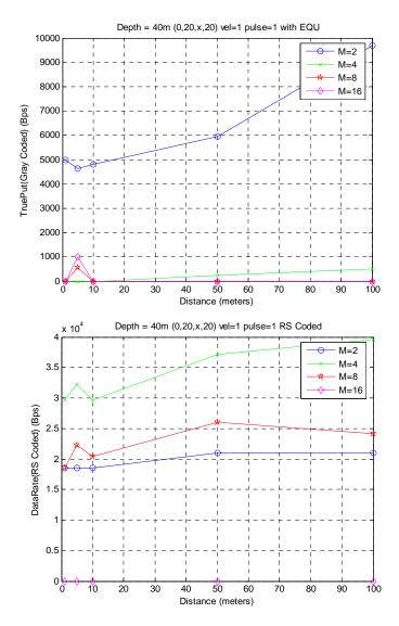
Figure 5.33: Trueput and RS coded data rate performance of the diver scenario#2 and boundary state scenario#1 with Doppler shift (v=1 m/sec)
