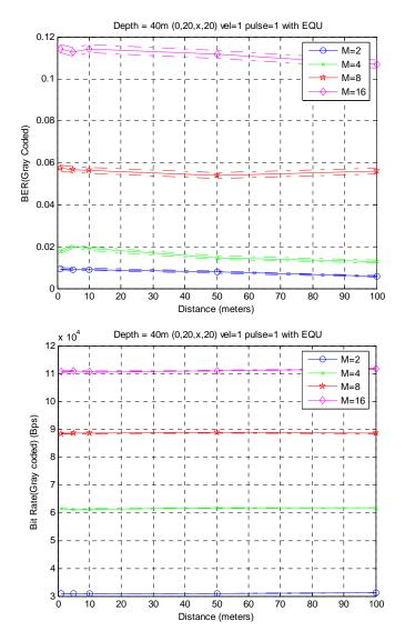
Figure 5.32: BER and bit rate performance of the diver scenario#2 and boundary state scenario#1 with Doppler shift (v=1 m/sec)
