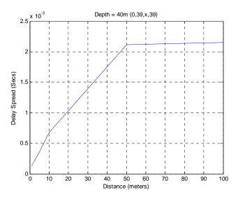
Figure 5.19: Delay Spread profile for diver scenario#1 and boundary state scenario#1
