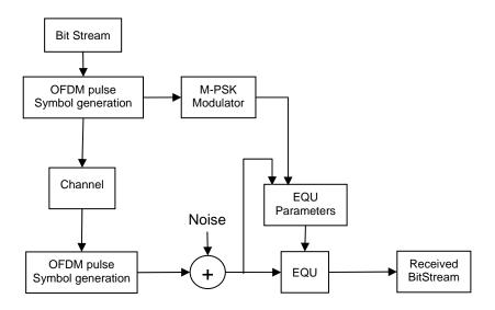
Figure 4.3: Equalization parameter selection and Equalization procedure
