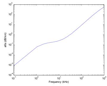
Figure 2.1: Absorption loss in Ocean at 20 °C and 35% salinity.
