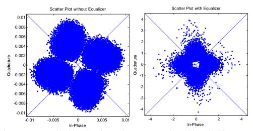
Figure 5.10: Received baseband complex representation with and without equalizer for underwater scenario of Diver#1@(0,39), Diver#2@(100,39) depth=40 m SS=0, porosity=0.2Noiseless and relative velocity v=1 m/sec, OFDM pulse length 1 msec, cyclic extension 5.4 msec
