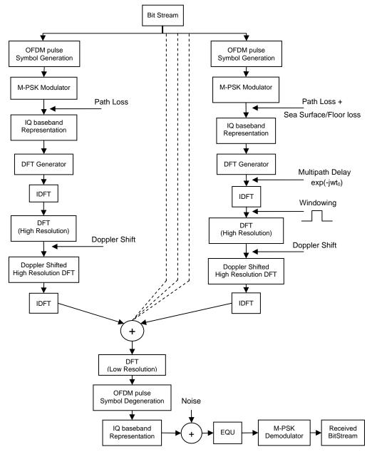
Figure 4.1: OFDM simulation procedure
