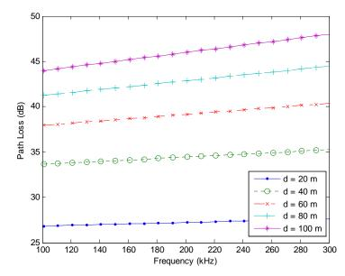
Figure 2.2: Total loss between 100 kHz and 300 kHz for several distances
