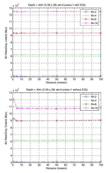
Figure 5.21: Bit rate performance of frequency domain equalized and nonequalized system
