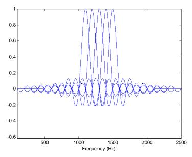
Figure 3.2: Spectra of carriers in OFDM symbol
