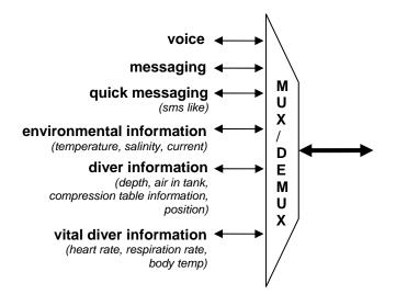
Figure 3.8: Architecture of the application layer
