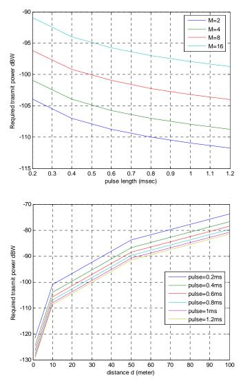
Figure 3.7: Required transmit power level to achieve the desired  $1 \times 10^{-3}$  BER for 300 kHz<sup>th</sup> symbol in OFDM pulse (a) with respect to pulse length at a distance of 10 m (b) with respect to distance for QPSK modulation.
