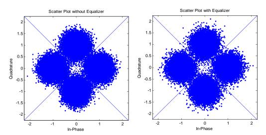
Figure 5.13: Received baseband complex representation with and without equalizer for underwater scenario of Diver#1@(0,39), Diver#2@(1,39) depth=40 m SS=0, porosity=0.2 Noisy and motionless case, OFDM pulse length 1 msec, cyclic extension 5.4 msec
