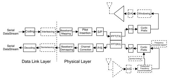
Figure 3.3: Block diagram of OFDM transceiver
