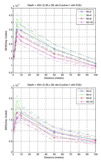
Figure 5.28: BER performance of the diver scenario#1 for boundary state scenario#1 and #2
