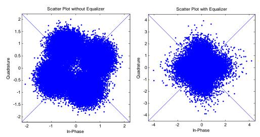
Figure 5.15: Received baseband complex representation with and without equalizer for underwater scenario of Diver#1@(0,50), Diver#2@(1,50) depth=100 m SS=0, porosity=0.2 Noisy and relative velocity v=1 m/sec, OFDM pulse length 1 msec, cyclic extension 5.4 msec
