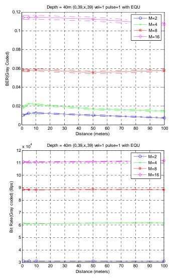
Figure 5.36: BER and bit rate performance of the diver scenario#1 and boundary state scenario#1 with Doppler shift (v=1 m/sec) and multipath
