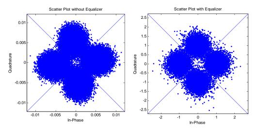
Figure 5.18: Received baseband complex representation with and without equalizer for underwater scenario of Diver#1@(0,39), Diver#2@(100,39) depth=40 m SS=0, porosity=0.2 Noisy and relative velocity v=1 m/sec case, OFDM pulse length 0.4 msec, cyclic extension 5.4 msec
