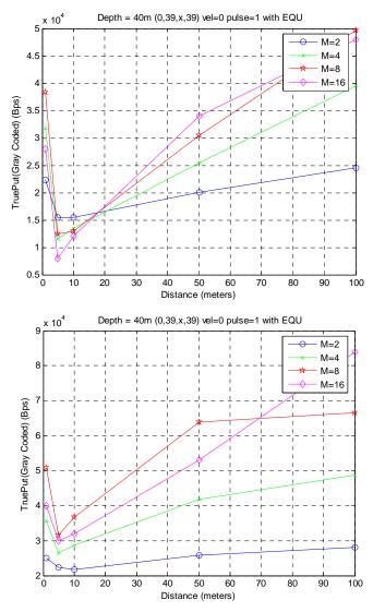
Figure 5.30: Trueput performance of the diver scenario#1 for boundary state scenario#1 and #2
