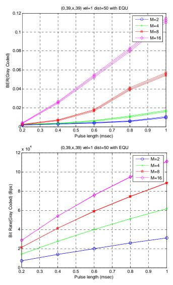
Figure 5.38: BER and bit rate performance of the diver scenario#1 and boundary state scenario#1 with Doppler shift (v=1 m/sec) and multipath with respect to OFDM pulse length
