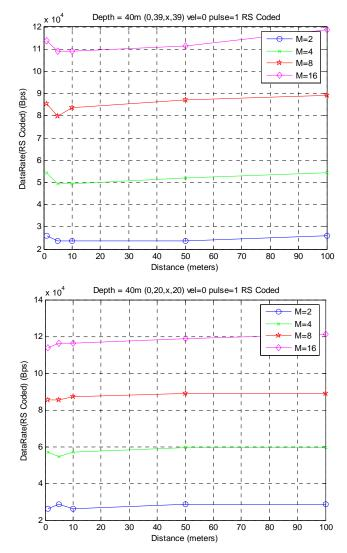
Figure 5.26: RS Coded data rate performance of the diver scenario#1 and #2
