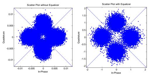
Figure 5.14: Received baseband complex representation with and without equalizer for underwater scenario of Diver#1@(0,39), Diver#2@(100,39) depth=40 m SS=0, porosity=0.2 Noisy and motionless case, OFDM pulse length 1 msec, cyclic extension 5.4 msec
