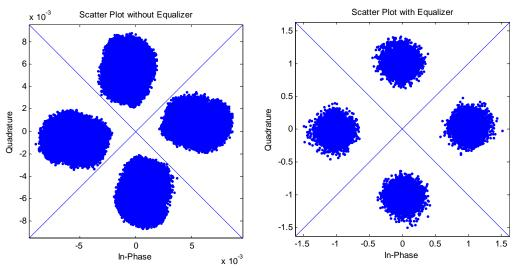
Figure 5.12: Received baseband complex representation with and without equalizer for underwater scenario of Diver#1@(0,39), Diver#2@(100,39) depth=40 m SS=0, porosity=0.2 Noiseless and relative velocity v=1 m/sec case, OFDM pulse length 0.4 msec, cyclic extension 5.4 msec
