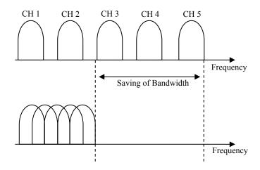
Figure 3.1: Comparison of FDM and OFDM.
