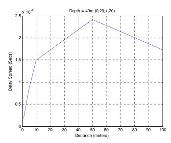
Figure 5.22: Delay spread profile of diver scenario#1 and #2 with boundary state scenario#1
