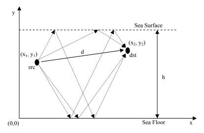
Figure 2.5: 5-Ray Underwater Acoustic Channel Model
