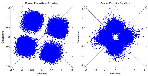
Figure 5.6: Received baseband complex representation with and without equalizer for underwater scenario of Diver#1@(0,50), Diver#2@(1,50) depth=100 m SS=0, porosity=0.2 Noiseless and relative velocity v=1 m/sec, OFDM pulse length 1 msec, cyclic extension 5.4 msec
