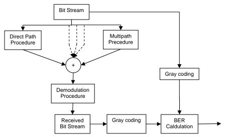
Figure 4.2: Gray coding and BER calculation simulation procedure
