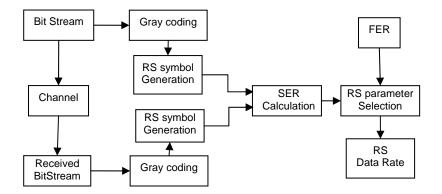
Figure 4.4: RS code parameter selection and RS coded data rate calculation procedure
