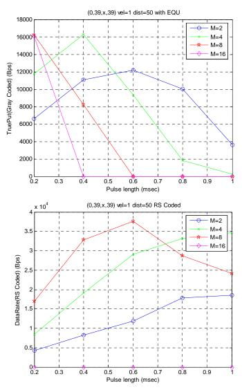
Figure 5.39: Trueput and RS coded data rate performance of the diver scenario #1 and boundary state scenario #1 with Doppler shift (v=1 m/sec) and multipath with respect to OFDM pulse length
