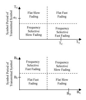
Figure 2.7: Characteristic of communication channel
