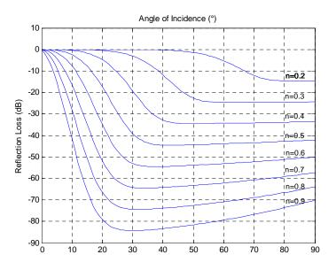
Figure 2.4: Sea floor loss at 200 kHz for several porosity values with respect to angle of incidence
