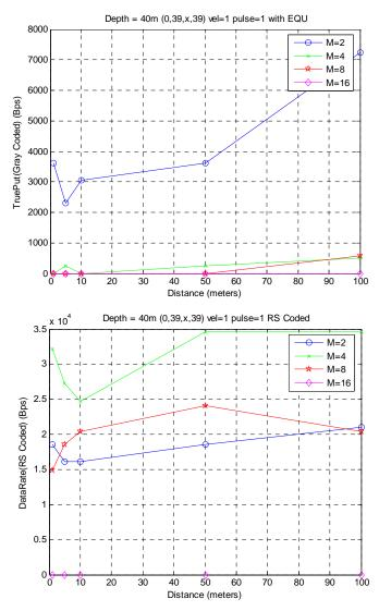
Figure 5.37: Trueput and RS coded data rate performance of the diver scenario#1 and boundary state scenario#1 with Doppler shift (v=1 m/sec) and multipath
