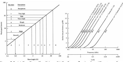
Figure 2.3: (a) Sea-State Conditions (b) Surface reflection loss (Courtesy of W.S. Burdic, Underwater Acoustic System Analysis, pp. 132-133)
