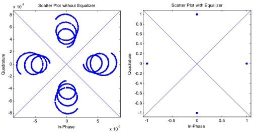
Figure 5.4: Received baseband complex representation with and without equalizer for underwater scenario of Diver#1@(0,39), Diver#2@(100,39) depth=40 m SS=0, porosity=0.2 Noiseless and motionless case, OFDM pulse length 1 msec, cyclic extension 5.4 msec
