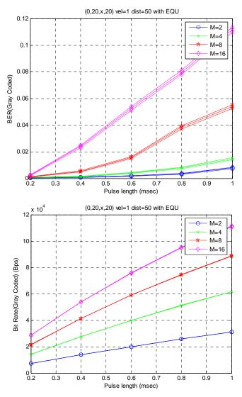
Figure 5.34: BER and bit rate performance of the diver scenario#2 and boundary state scenario#1 with Doppler shift (v=1 m/sec) with respect to OFDM pulse length
