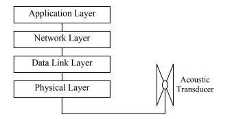
Figure 1.1: Layered architecture of underwater acoustic communication system
