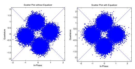
Figure 5.16: Received baseband complex representation with and without equalizer for underwater scenario of Diver#1@(0,50), Diver#2@(1,50) depth=100 m SS=0, porosity=0.2 Noisy and relative velocity v=1 m/sec case, OFDM pulse length 0.4 msec, cyclic extension 5.4 msec
