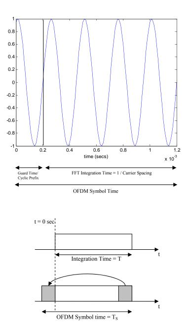
Figure 3.4 (a) Cyclically extended OFDM pulse (b) Cyclic Extension
