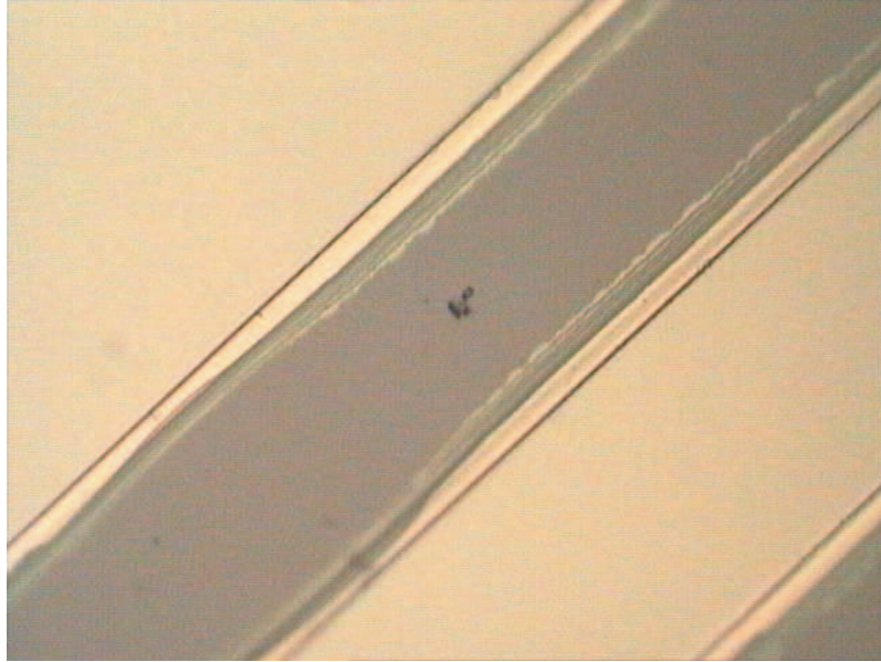
Figure 3.5: The undercutting problem in the fabrication of beam process
