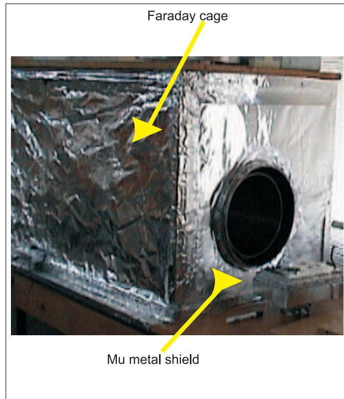
Figure 5.8: Faraday cage made with aluminium sheet of thickness of about 0.5 mm to shield against high frequency EM waves.
