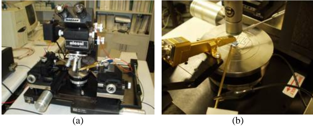
Figure 3.10: (a) The probe station. With the help of objectives, we can make contact to the pads of the photodetectors. (b) The sample on the probe station, where two DC probes touch the pads, while the active area is illuminated with the fiber.
