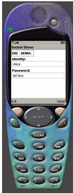
Figure 14 KToolbar Simulator: KToolbar is a mobile phone simulator, where developer may run their MIDP (Mobile information device profile) applications.
