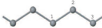
Figure 4.15: Initial zigzag structure with \widehat{123} = 120^\circ . The optimized Si3 has zigzag structure with bond lengths d_{12} = d_{23} = 2.18\text{\AA} , d_{13} = 3.74\text{\AA} , angle \widehat{123} = 118.22^\circ , and binding energy E_{binding} = 3.85eV . C3 structure disintegrated after optimization.
