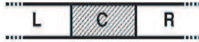
Figure 3.5: A conductor described by the Hamiltonian H_C , connected to leads L and R , through the coupling matrices h_{LC} and h_{CR} .
