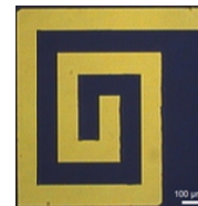
Fig. 1. Top-view micrograph of our fabricated bioMEMS sensor.
