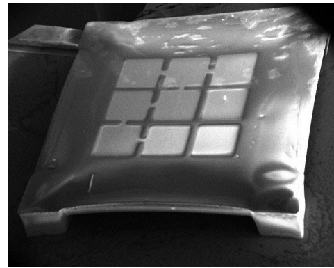
Fig.8. Angled-view SEM micro-graph of a completed MRA
