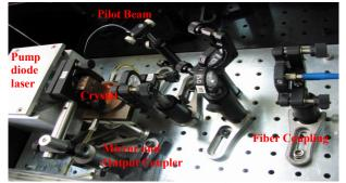
Figure 1: Tm:YAP laser setup and its components
