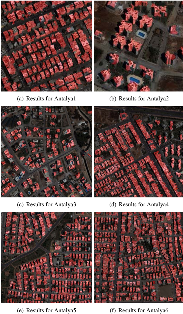
Fig. 4. Building detection results. The detected buildings are highlighted in red.
