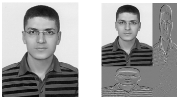
Fig. 3. Example image (left) and 2-D unbalanced lifting wavelet transformed image with p=3:2 and q=3:1 (right). Highband subimages are amplified by a factor of five.
