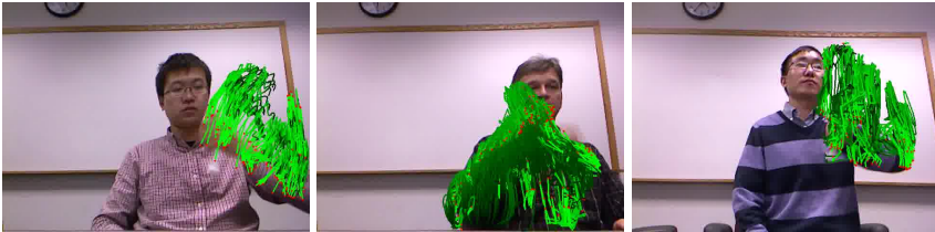
Fig. 5. Regardless of whichever direction user shakes the inhaler device, we get many long trajectories as the result.
