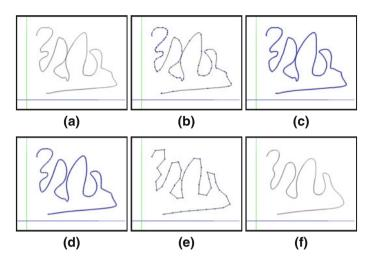
Fig. 3 a Initial user input. b Non-uniform distribution (706 points). c Re-sampled (2877 points). d Gaussian filtered. e Reverse Chaikin subdivided (47 points to *represent*). f Final B-spline curve (188 points to *render*)
