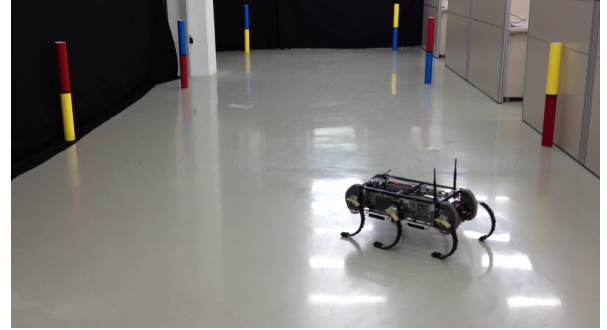
Fig. 12. A snapshot from the experimental setup in its initial state. Six colored landmarks are scattered throughout the environment, observable through a camera mounted on the RHex robot.
