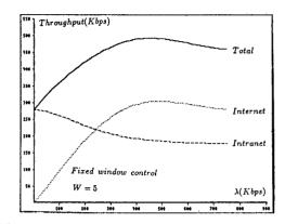
Figure 3: Throughput of a network versus internetwork load
