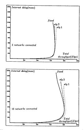
Figure 8: Average internet delay versus total throughput for different number of networks connected to internetwork
