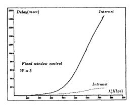
Figure 4: Average message delay versus internetwork load
