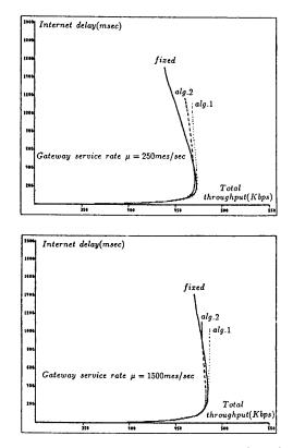
Figure 10: Average internet delay versus total throughput for different gateway service rates
