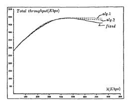
Figure 5: Total throughput versus internetwork load
