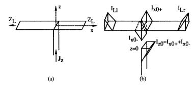
Fig.1. (a) Microstrip line fed by a probe and terminated in complex impedances, and(b) discontinuous expansion functions at the source and load junctions.
