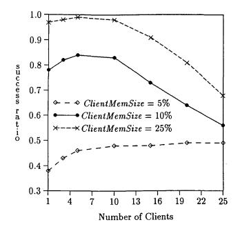
Figure 2: Performance with different client memory sizes (NetworkBandwidth = 8 Mbps).
