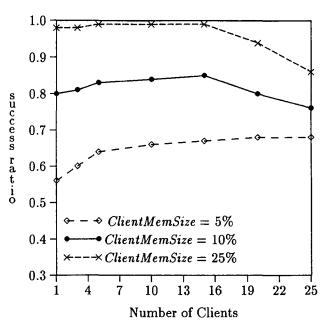
Figure 3: Performance with different client memory sizes (NetworkBandwidth = 80 Mbps).
