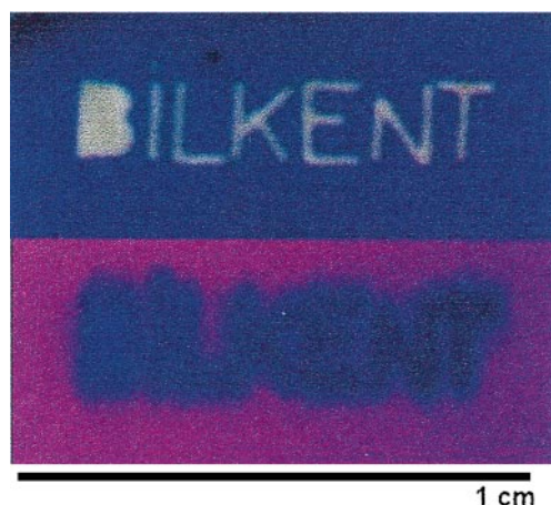
Fig. 7. Photographs of a macroscale lithographic example of a PVC film containing methyl violet (lower field) and methyl violet and hydroquinone (upper field)
