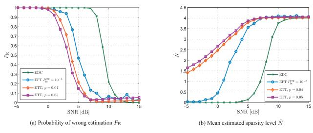
Fig. 1: Probability of wrong estimation  $P_{\rm E}$  (a) and estimated sparsity  $\hat{N}$  (b) as functions of the SNR for T=M
