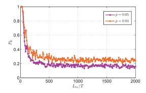
Fig. 3: Probability of wrong estimation  $P_{\rm E}$  as a function of L for T=M,  ${\rm SNR}=5~{\rm dB}$
