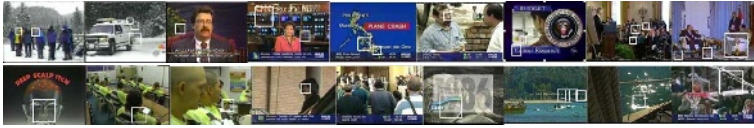
Fig. 2. Examples to the false detections eliminated by using top : the average skin color, bottom : the number of skin pixels
