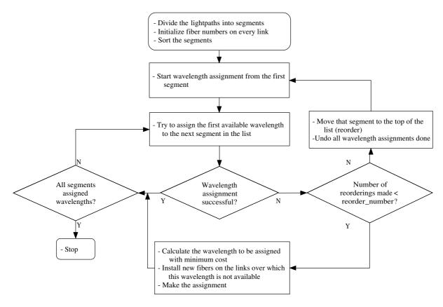
Fig. 2. Flowchart of the RLPF wavelength assignment algorithm
