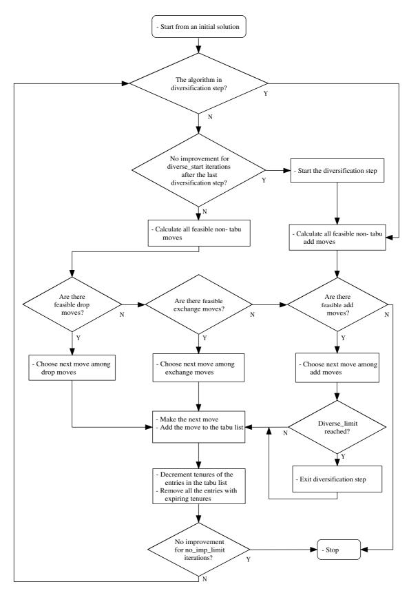
Fig. 3. Flowchart of the TSCP algorithm
