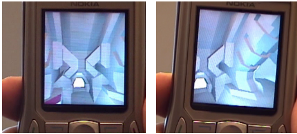
Fig. 1. A 3D virtual environment. The user can move the device up, down, left and right to look around the space. Mapping physical motion to viewing direction in the space creates the illusion of a small window into an environment that surrounds the user.
