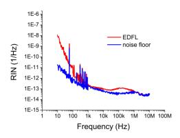
Figure 4: Relative intensity noise (RIN) of the EDFL, along with the measurement noise floor.
