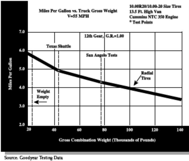
Fig. 1. Miles per Gallon versus vehicle weight [22]
