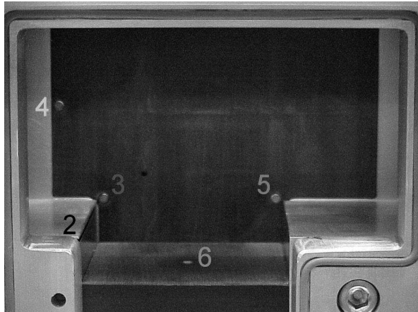
Fig. 3. The locations of the pressure transducers placed in the test section
