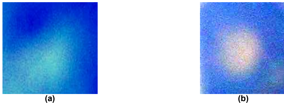
Figure 1: Pictures of 10 μm thick acrylic solgel film embedded with (a) 21 nm and (b) 6 nm TiO 2 nanoparticles that are contaminated with the same methylene blue solution and activated under the same conditions.
