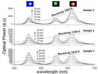
Figure 2. Luminescence spectra of our nanocrystal hybridized warm-white LEDs (Samples 1-3) when electrically driven at room temperature.
