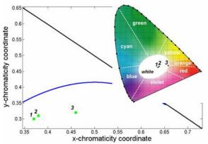
**Figure 1.**Tristimulus coordinates of our nanocrystal-hybridized warm-white LEDs (Samples 1, 2 and 3 shown in green points 1, 2 and 3) along with the planckian locus (shown in blue line). The inset shows these tristimulus coordinates on a CIE 1931 chromaticity diagram.
