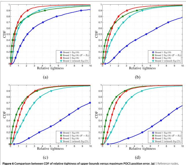
**Figure 6** Comparison between CDF of relative tightness of upper bounds versus maximum POCS position error. (a) 5 Reference nodes, (b) 10 reference nodes, (c) 15 reference nodes, and (d) 20 reference nodes.
