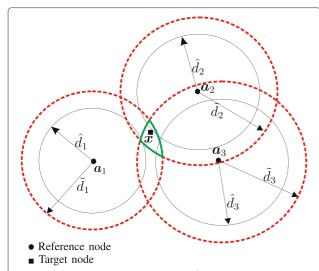
Figure 3 Every distance measurement  $\hat{d}_i$  is replaced by a larger value  $\tilde{d}_i$ . The intersection drawn by green color now definitely contains the target node position.
