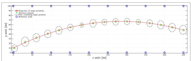
**Figure 8 Confidence discs formed by POCS estimates and corresponding upper bounds (Bound 2, Equation 18).** Discs contain the location of a target moving according to a trajectory.
