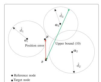
**Figure 2** The intersection is empty and measurement one has a positive error. The actual error and an upper bound on the position error are shown in this figure.
