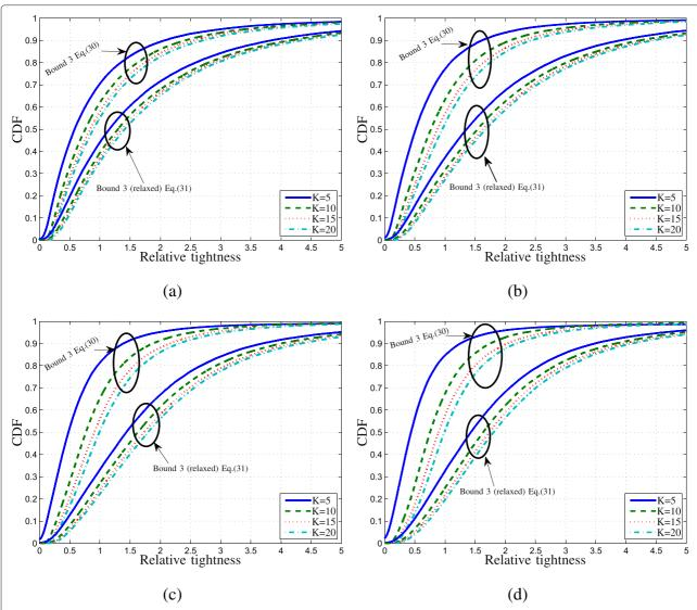
**Figure 7 CDF of relative tightness for Bound 3 and Bound 3 (relaxed) for different numbers of distance estimates for every link, K.** (a) 5 Reference nodes, (b) 10 reference nodes, (c) 15 reference nodes, and (d) 20 reference nodes.
