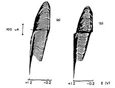
Fig. 2. Cyclic voltammogram of pyrrole in acetonitrile on a) bare Pt b) polyimide coated Pt electrodes.
