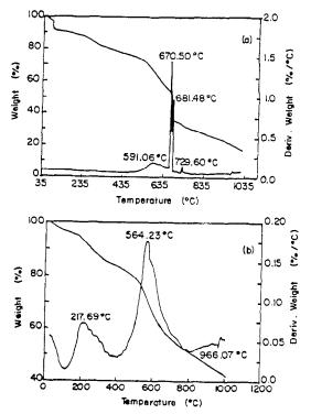
Fig. 3. Thermal Gravimetric Analysis a) PI/PPy electrolytic film b) mechanical mixture of PI and PPy.
