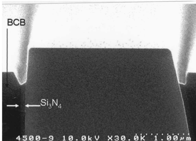
FIG. 5. Cross-sectional SEM picture of InP devices with \text{Si}_3\text{N}_4 sidewall protection. Note that the top \text{Si}_3\text{N}_4 layer is etched away during BCB etch.
