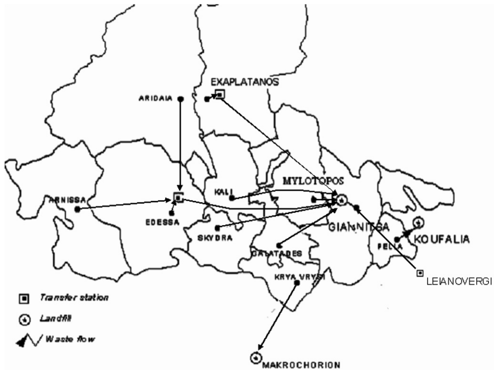
Fig. 6. MSW management of the prefecture of Pella in accordance with the best compromise solution for the region of Central Macedonia, where the inter-prefectural collaboration of the prefecture of Pella with the prefecture of Imathia (with waste flows from Platy to Leianovergie and from Krya Vrisi to Makrochorion) is also illustrated.
