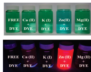
Figure 4. Digital photographs of the chemosensor solutions ( 5.0 \mu\text{M} ) in the presence of different metal ions at 100 \mu\text{M} concentration. The upper plate is taken under ambient light, and the bottom one under UV illumination at 360 nm. Solvent: ethanol–aqueous buffer mixture (5% in ethanol, HEPES 0.1 M, pH = 7.2).
