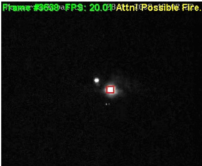
Fig. 7. Correct alarm for a fire at night and elimination of fire-truck headlights.
