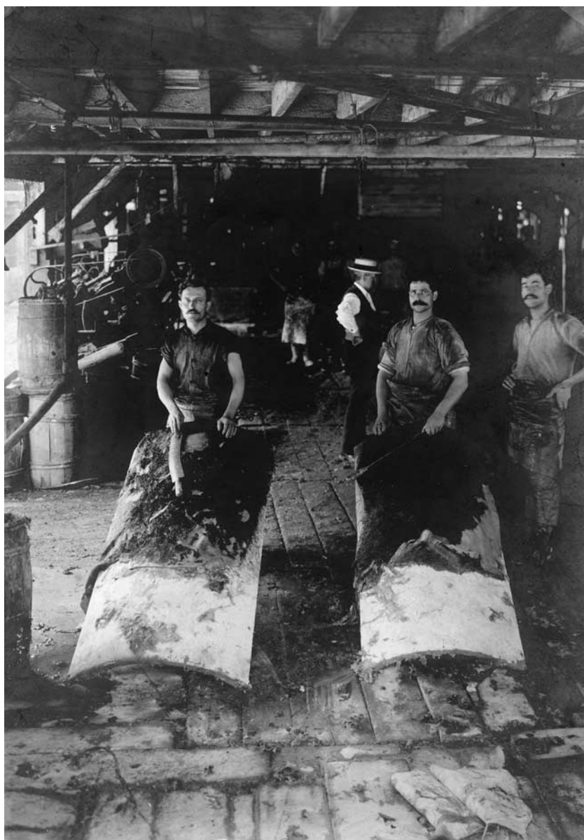
Figure 2. An image from J.A. Lord Jr leather shop's beam house in 1906. These three leatherworkers were identified in the original picture as Big Greek, Greek M., and Greek D. The hides were spread across a wooden beam and the hair or flesh, fat, and muscle were shaved off. The process is called de-hairing or de-fleshing. Information about the picture is provided in Ted Quinn, Peabody's Leather Industry (Charleston, SC, 2008), p. 12. From the archives of Peabody Historical Society, Peabody, MA; reproduced with permission.
