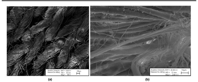
Figure 4. SEM images of 14% SeaCell Active/86% cotton blended fabric. a) unwashed; b) 20 times washed
