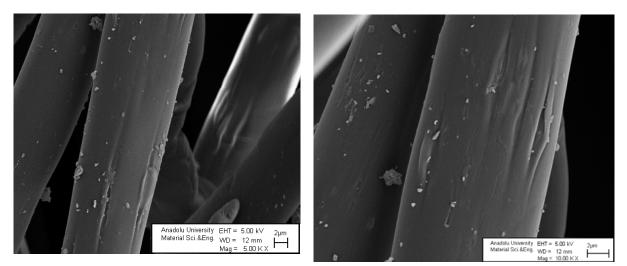
Figure 2. SEM images of SeaCell Active fibers (magnified 5,000 and 10,000 times)
