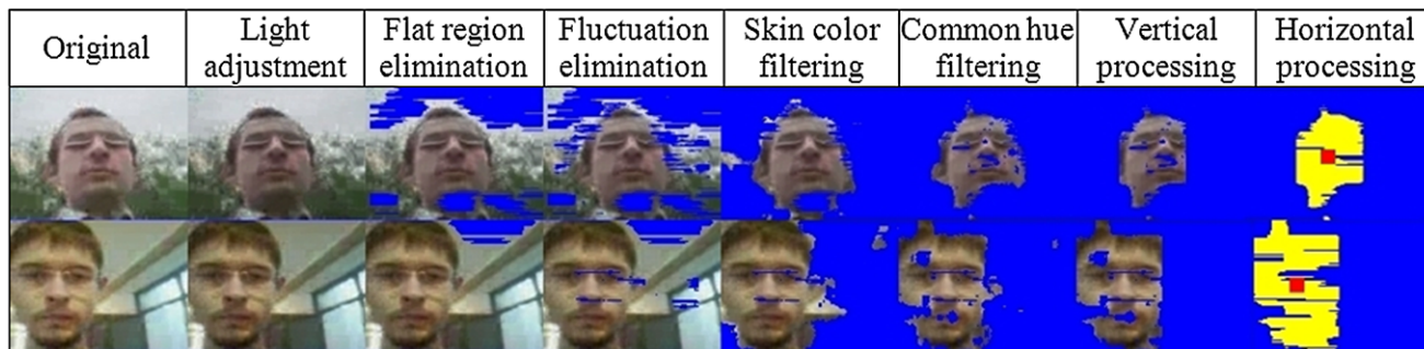
Fig. 12 Step by step execution of the algorithm on two different samples. (For a better demonstration of the steps, the whole image is scanned without clipping)
