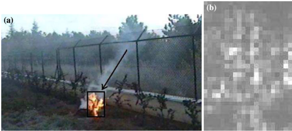
Fig. 8. (a) Fire, and (b) the absolute sum of spatial wavelet transform coefficients, |I_{lh}(k,l)| + |I_{hl}(k,l)| + |I_{hh}(k,l)| , of the region bounded by the indicated rectangle.
