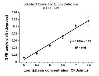
Figure 6 | Validation with *E. coli* spiked in peritoneal dialysis (PD) fluid. The concentration range of  $10^5$  CFUs/mL to  $3.2 \times 10^7$  CFUs/mL was evaluated. At each concentration, 6 microchips were evaluated at 5  $\mu$ L/minute for 20 minutes. The linear curve shows the least squares fit with  $R^2 = 0.98$  (n = 6, error bars represent standard error of the mean).
