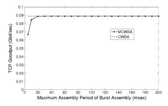
Fig. 11 TCP performance of CWBA and MCWBA algorithms (pessimistic case) in the linear OBS network topology
