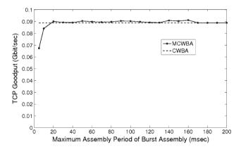
Fig. 9 TCP performance of CWBA and MCWBA algorithms (average of 5 simulations) in the linear OBS network topology
