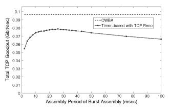
Fig. 6 TCP performance of timer-based and CWBA algorithms in the mesh OBS network topology
