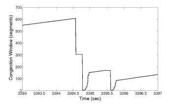
Fig. 5 Congestion window evolution of timer-based assembly algorithm with an assembly delay of 8 ms for TCP Reno
