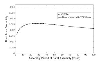
Fig. 7 Burst loss probabilities for timer-based and CWBA algorithms in the mesh OBS network topology
