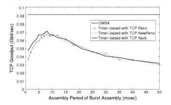
Fig. 3 Performance of timer-based and CWBA algorithms for the linear OBS network topology
