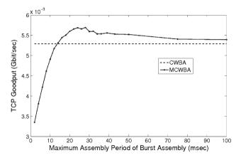
Fig. 13 TCP performance of CWBA and MCWBA algorithms for the 4th TCP flow for the mesh OBS network topology
