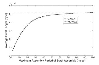
Fig. 15 Average burst lengths for CWBA and MCWBA algorithms in the mesh OBS network topology
