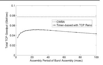
**Fig. 18** TCP performance of timer-based and CWBA algorithms in the mesh OBS network topology with dynamic flows ( $t \in [5000, 10000)$  s)
