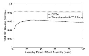
Fig. 16 TCP performance of timer-based and CWBA algorithms in the mesh OBS network topology with dynamic flows ( $t \in [0, 10000)$  s)
