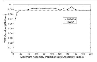
Fig. 10 TCP performance of CWBA and MCWBA algorithms (optimistic case) in the linear OBS network topology
