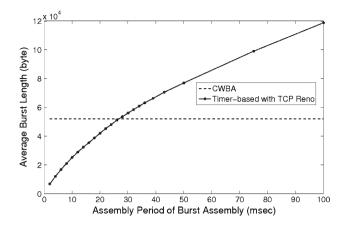
Fig. 8 Average burst lengths for timer-based and CWBA algorithms in the mesh OBS network topology
