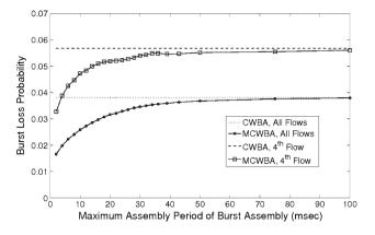
Fig. 14 Burst loss probabilities for CWBA and MCWBA algorithms in the mesh OBS network topology
