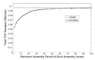
Fig. 12 TCP performance of CWBA and MCWBA algorithms for the mesh OBS network topology
